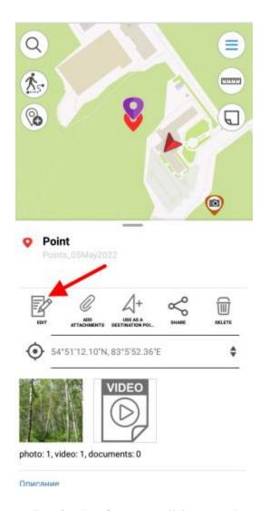
Being in the feature editing mode, you can change the feature geometry. To delete the point, tap it on the map. To add the new point, tap the empty place on the map. To move the point, select it on the map and drag it to required place on the map.
