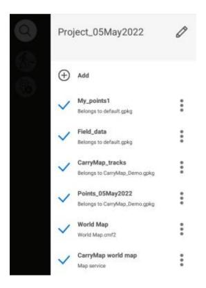
To turn off layer visibility, tap 'near the required layer name and the icon will change its color to grey '. Note that the layer will not be deleted from the project, it just will not be shown on the map. To turn the hidden layer on, tap the icon near its name again.
