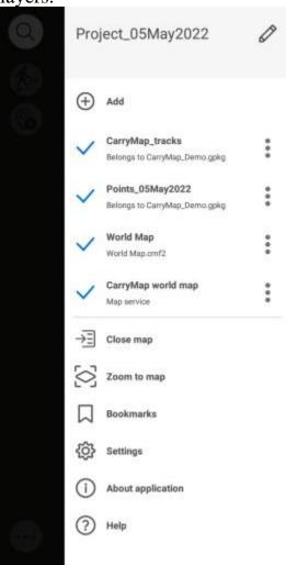
If the layer is the first one in the list, it will be displayed on top of all layers on your map, accordingly. To zoom to layer in the project, tap the three dots menu and select *Zoom to layer*.
