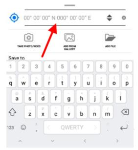
You can change coordinates format, if needed. To do so, select the feature and in the appeared identification window tap the line with coordinates to change the format.
