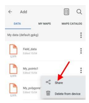
When sharing gpkg layer you can select the format: SHP, KMZ, GPKG, GPX.
