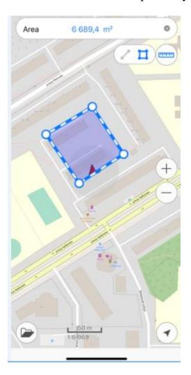
To delete the needless point, tap it again. The calculated distance or area will be shown in the upper part of the measurement window.
